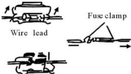
Insert the fuse and keep it securely in place
