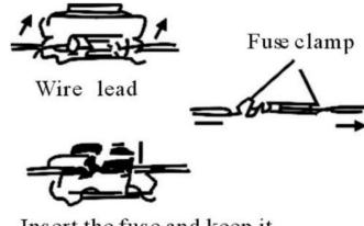
Insert the fuse and keep it securely in place
